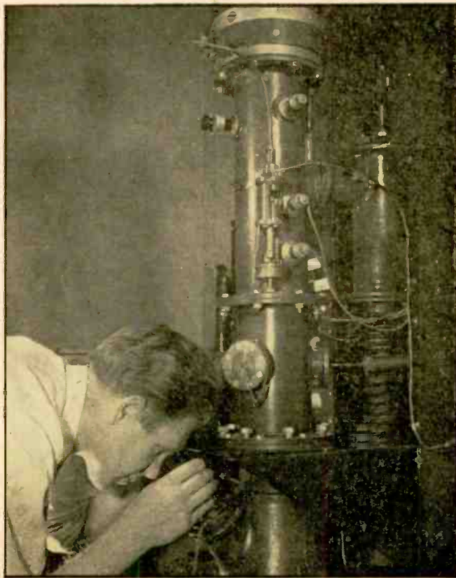
Dr. Gulbransen inspects the target of his "machine-gun." This three feet of steel pipe is a genuine electron tube, in spite of the fact that it resembles a section of water main more closely than it does one of the tubes in your radio. The associated apparatus is used to maintain the vacuum and control the admixture of traces of desired gases, when required.
